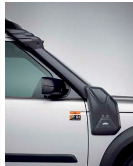
Raised Air Intake ADL780010
