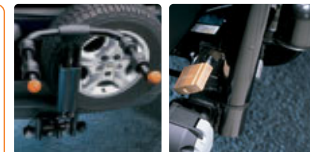
Bike carrier shown with padding to prevent damage to both vehicle and bikes
